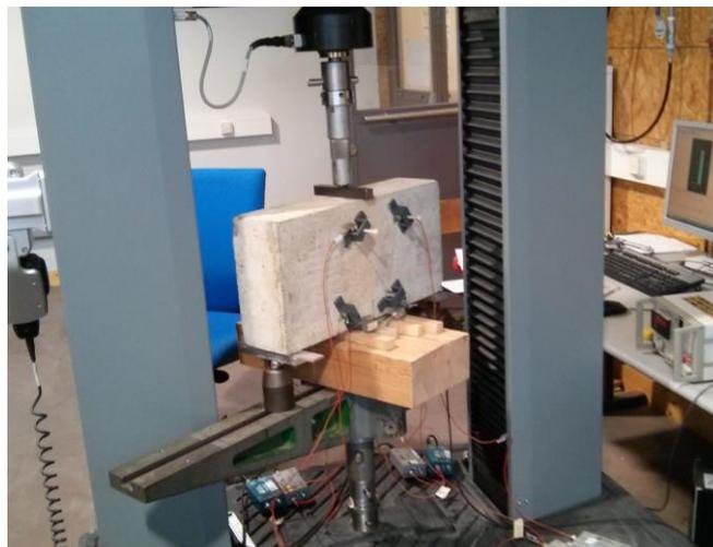
**Figure 1.** Essai de flexion 3 points.
