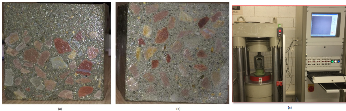
Figure 5. (a) Concrete specimens 70 \times 70 \times 280 mm with and (b) without aggregate segregation along the depth direction, (c) Experimental Set-up for the uniaxial compression test on specimens of mortar to obtain the mechanical behavior.
